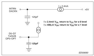
Figure 17. Test Conditions on Outputs
