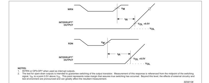
Figure 10. Interrupt Timing (80xxx mode)
