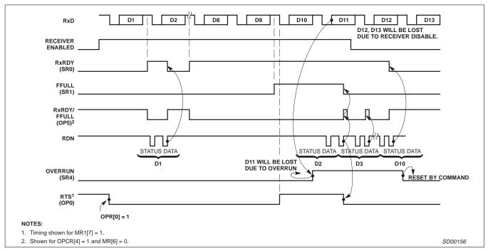
Figure 15. Receiver Timing
