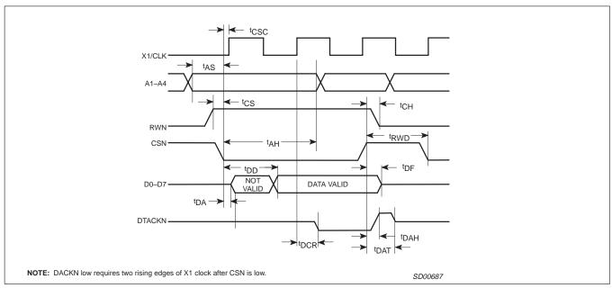
Figure 6. Bus Timing (Read Cycle) (68XXX mode)
