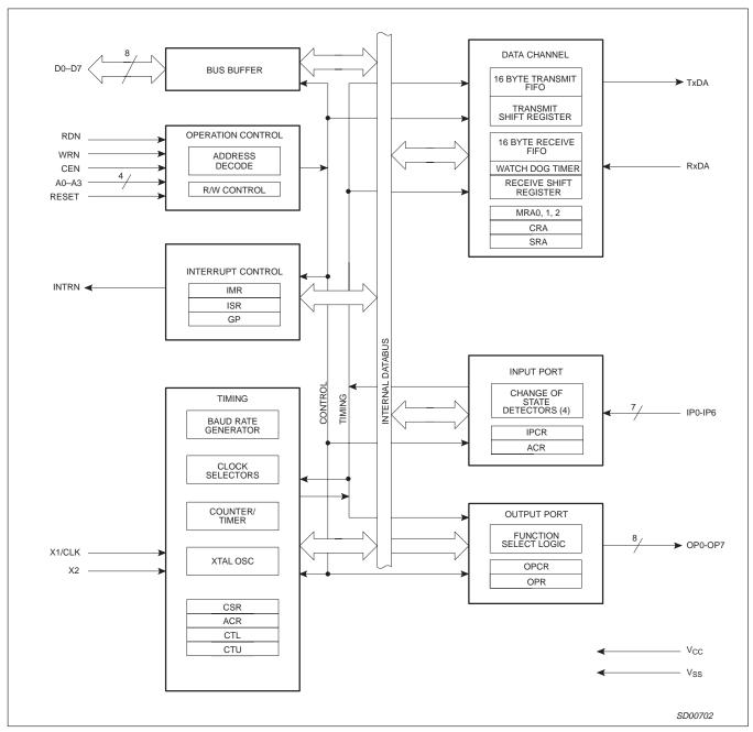
Figure 1. Block Diagram (80XXX mode)
