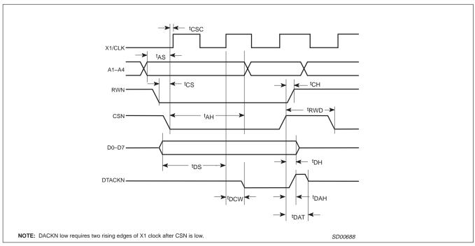
Figure 7. Bus Timing (Write Cycle) (68XXX mode)
