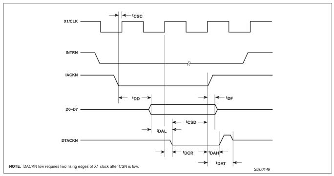
Figure 8. Interrupt Cycle Timing (68XXX mode)
