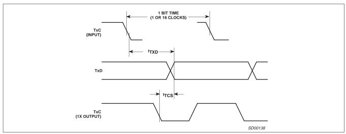
Figure 12. Transmitter External Clocks
