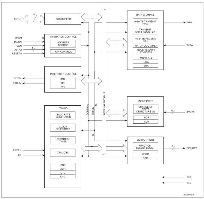
Figure 2. Block Diagram (68XXX mode)
