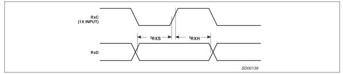
Figure 13. Receiver External Clock
