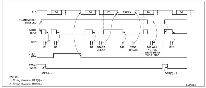
Figure 14. Transmitter Timing
