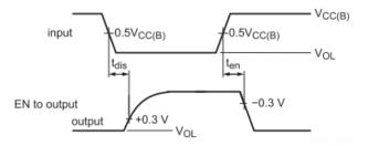
Figure7: Propagation Delay and Enable and disable time
