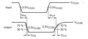
Figure 5: Propagation Delay and Transition Times B→A
