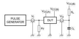
$R_L = load resistor; 1.35 k\Omega on port B$
