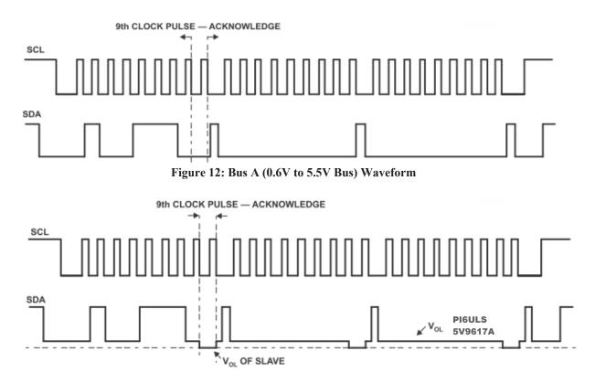
Figure 13: Bus B (2.2V to 5.5V Bus) Waveform
