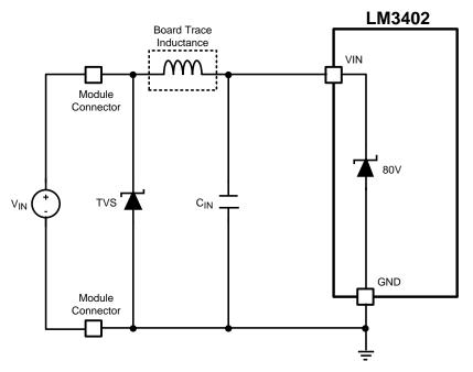
Figure 26. VIN Pin With Typical Input Protection
