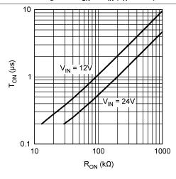
Figure 10.  $T_{ON}$  vs  $R_{ON}$ , LM3402 ( $T_A = 25$ °C)
