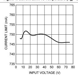
Figure 6. Current Limit vs  $V_{IN}$ , LM3402HV ( $T_A = 25$ °C)
