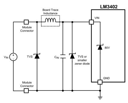
Figure 27. VIN Pin With Additional Input Protection
