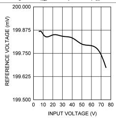
Figure 3.  $V_{REF}$  vs  $V_{IN}$ , LM3402HV ( $T_A = 25$ °C)
