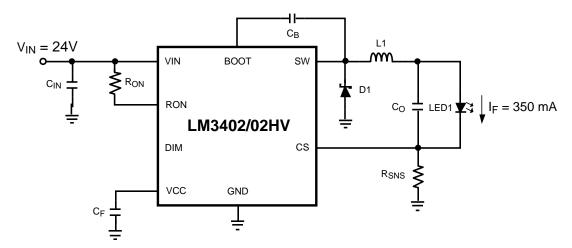
Figure 28. Schematic for Design Example 1
