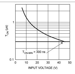
Figure 7.  $T_{ON}$  vs  $V_{IN}$ ,  $R_{ON}$  = 100 k $\Omega$  ( $T_A$  = 25°C)
