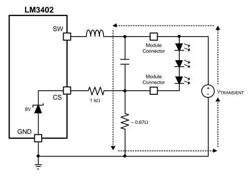
Figure 23. CS Pin, Transient Path With Protection
