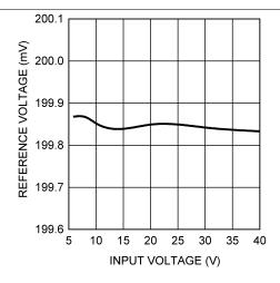
Figure 2.  $V_{REF}$  vs  $V_{IN}$ , LM3402 ( $T_A = 25$ °C)
