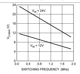
Figure 13.  $V_{O-MAX}$  vs  $f_{SW}$ , LM3402 ( $T_A = 25$ °C)
