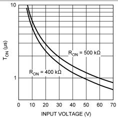
Figure 9.  $T_{ON}$  vs  $V_{IN}$ ,  $(T_A = 25^{\circ}C)$
