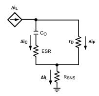
Figure 20. LED and Co Ripple Current
