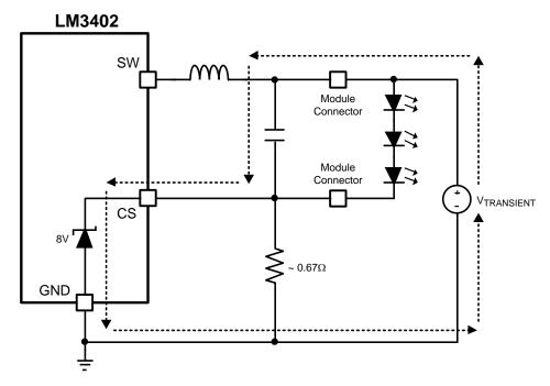
Figure 22. CS Pin. Transient Path
