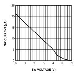
Figure 21. LED Current From SW Pin
