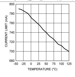
Figure 4. Current Limit vs Temperature (V<sub>IN</sub> = 24 V)
