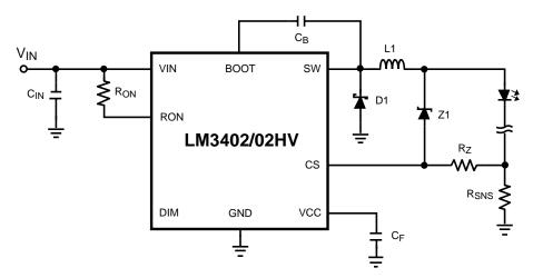
Figure 18. Output Open Circuit Protection
