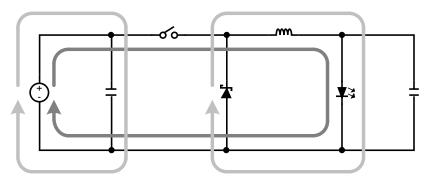
Figure 31. Buck Converter Current Loops
