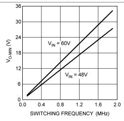
Figure 16.  $V_{O-MIN}$  vs  $f_{SW}$ , LM3402HV ( $T_A = 25$ °C)
