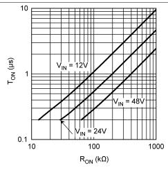
Figure 11.  $T_{ON}$  vs  $R_{ON}$ , LM3402HV ( $T_A = 25$ °C)
