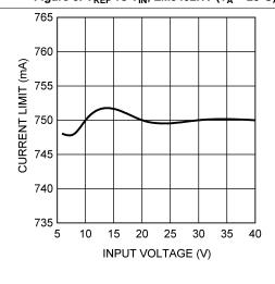
Figure 5. Current Limit vs  $V_{IN}$ , LM3402 ( $T_A = 25$ °C)
