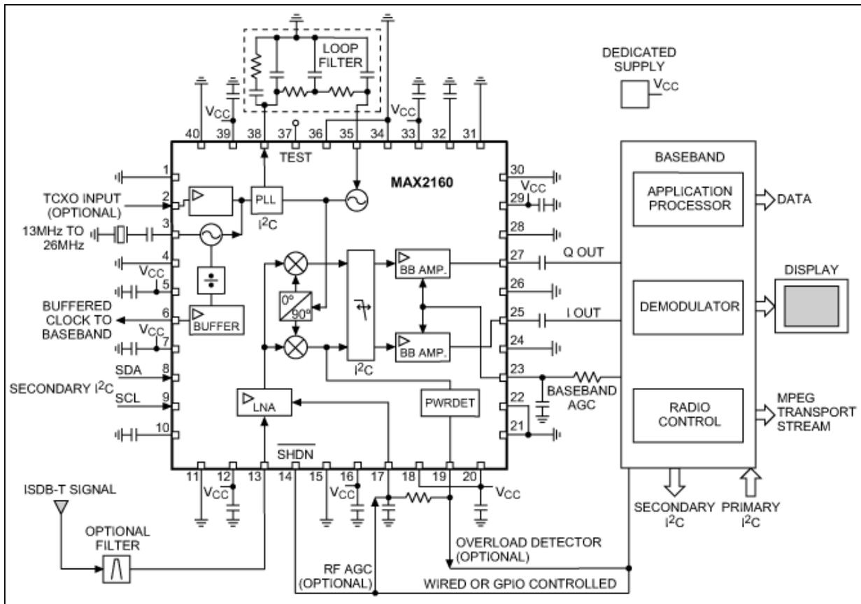
Figure 1. Diagram of a radio based on the MAX2160 tuner and a generic baseband processor.
