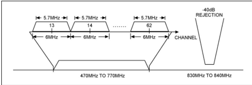
Figure 2. Illustration of the channelization process with the MAX2160 tuner.
