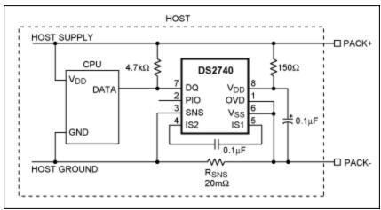
Figure 1. DS2740 installed in the host system.
