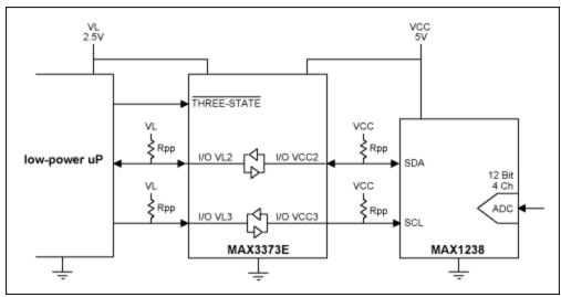
Figure 6. MAX3373E dual level translator used in an IIC-bus application with optional pull-up resistors Rpp.
