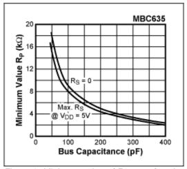
Figure 8. Minimum value of R<sub>P</sub> as a function of supply voltage with the value of R<sub>S</sub>as a parameter, from I<sup>2</sup>C-specification.
