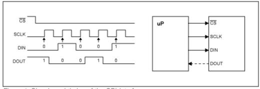
Figure 1. Signals and timing of the SPI-interface.
