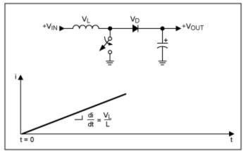
Figure 5. Charging phase: when the switch closes, current ramps up through the inductor.
