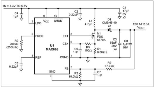
Figure 10. The MAX668 for current-mode-controlled boost circuit.
