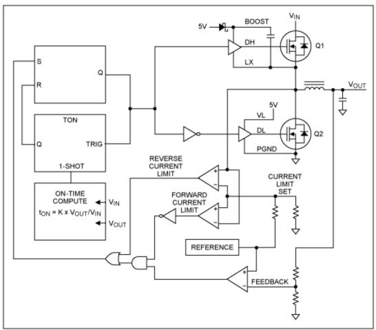
Figure 11. Simplified block diagram of Maxim's Quick-PWM control.
