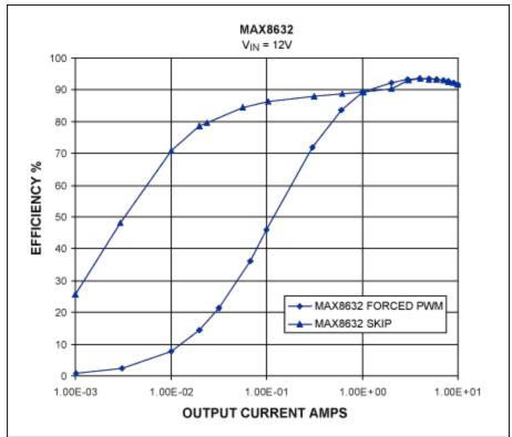
Figure 15. Efficiency with and without skip mode.
