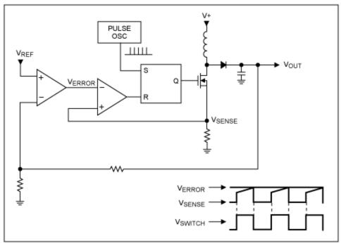
Figure 9. Current-mode pulse-width modulation.
