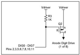
Figure 1. Current boosting the digit drive while retaining a low voltage LED supply.
