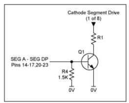
Figure 4. Current boosting the segment drive.
