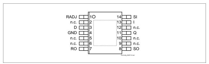
Figure 3 Pin configuration (top view)
