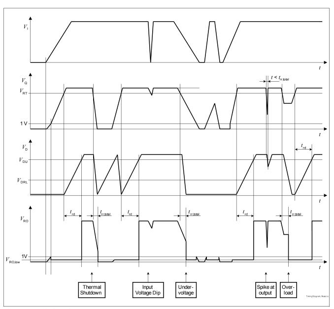
Figure 6 Timing diagram reset
