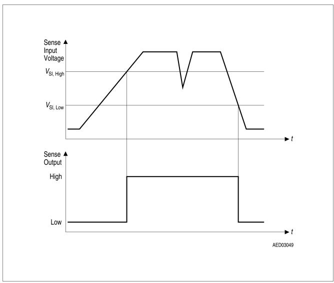
Figure 7 Sense timing diagram
