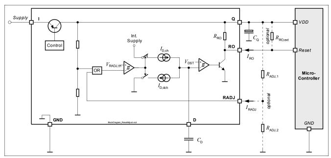
Figure 5 Block diagram reset function
