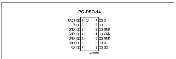
Figure 2 Pin configuration (top view)
