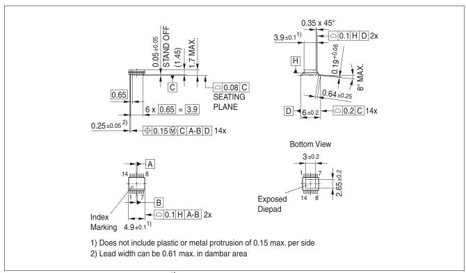
Figure 12 PG-SSOP-14 exposed pad<sup>1)</sup>
