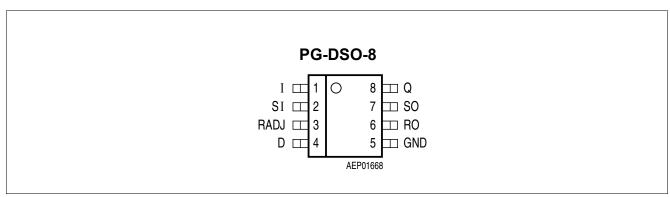
Figure 1 Pin configuration (top view)
