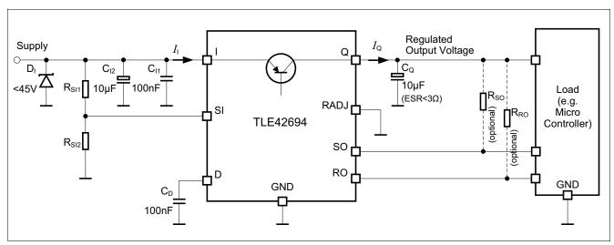
Figure 8 Application diagram with selecting default reset thresholds
