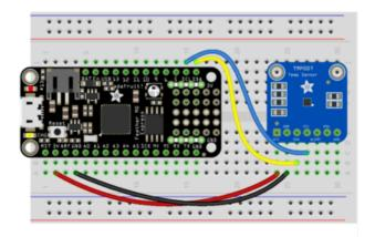
Board 3V to sensor VCC Board GND to sensor G Board SCL to sensor SCL Board SDA to sensor SDA
