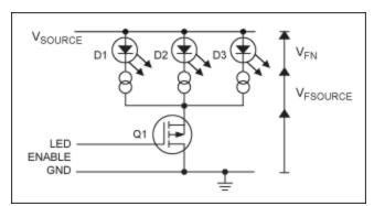
Figure 6. LED biasing with current sources.
