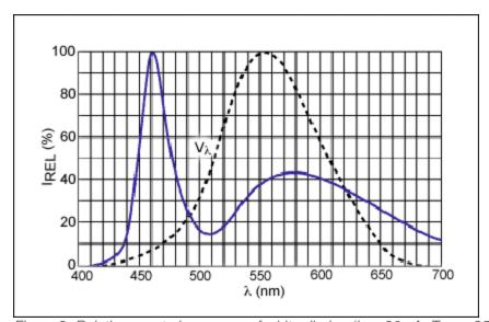
Figure 2. Relative spectral response of white diodes ( $I_F = 20mA$ ,  $T_A = +25$ °C).
