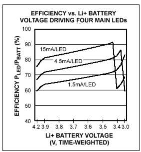
Figure 10. MAX1576 efficiency at typical lithium-battery voltages.
