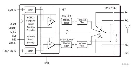
Figure 1. SKY77547 Functional Block Diagram
