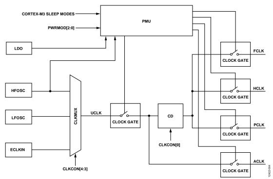
Figure 3. System Clock Architecture Block Diagram
