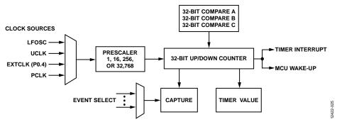
Figure 25. Wake-Up Timer Block Diagram
