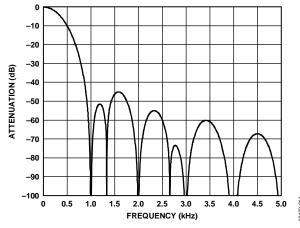
Figure 14. Modified Sinc3 Digital Filter Response at  $f_{ADC} = 1.0 \text{ kHz}$  (ADCFLT = 0x0087)
