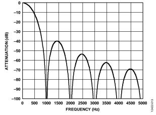
Figure 13. Typical Digital Filter Response at  $f_{ADC} = 1.0 \text{ kHz}$  (ADCFLT = 0x0007)
