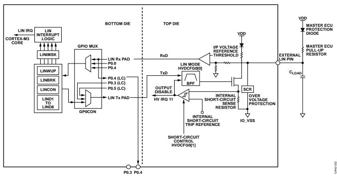
Figure 32. LIN Block Diagram
