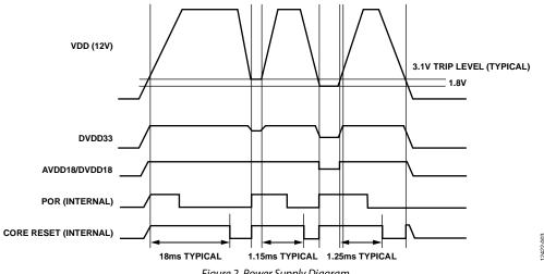
Figure 2. Power Supply Diagram
