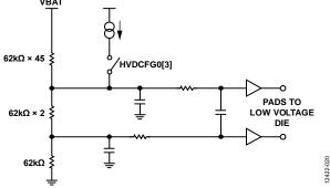
Figure 20. ADC1 Example Circuit Using Diagnostic Current Source on HV Die
