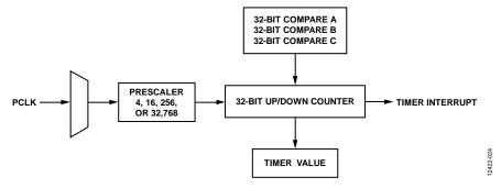
Figure 24. General-Purpose Timers Block Diagram
