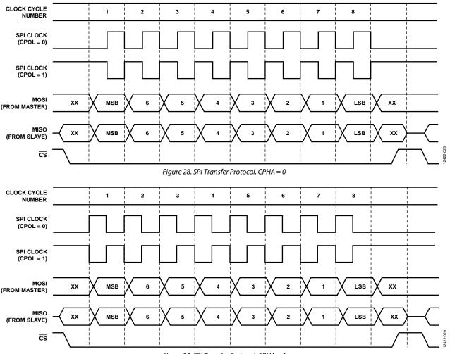
Figure 29. SPI Transfer Protocol, CPHA = 1
