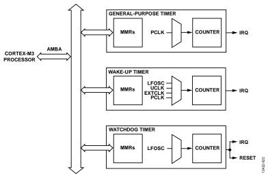
Figure 22. Timer Synchronization Block Diagram
