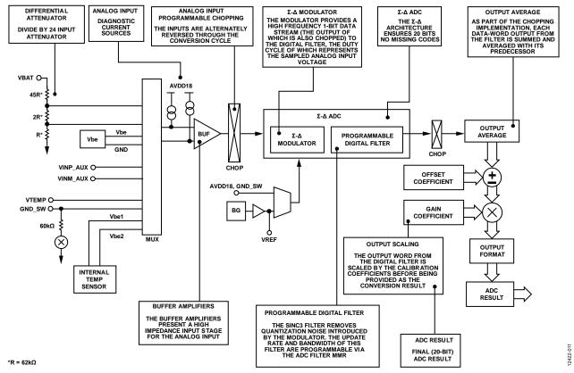
Figure 11. Voltage/Temperature ADC Top Level Overview
