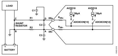
Figure 19. ADCO Example Circuit Using Diagnostic Current Sources
