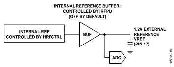
Figure 18. ADC Reference Configuration
