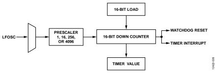
Figure 26. Watchdog Timer Block Diagram
