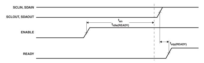
Figure 7.  $t_{stp(READY)}$  That Can Occur After  $t_{en}$  and  $t_{idle(READY)}$
