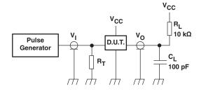
R<sub>L</sub> = Load resistor
