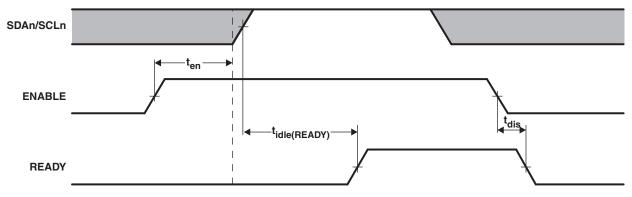
Figure 5. Timing for  $t_{\text{en}},\,t_{\text{idle(READY)}},\,\text{and}\,\,t_{\text{dis}}$
