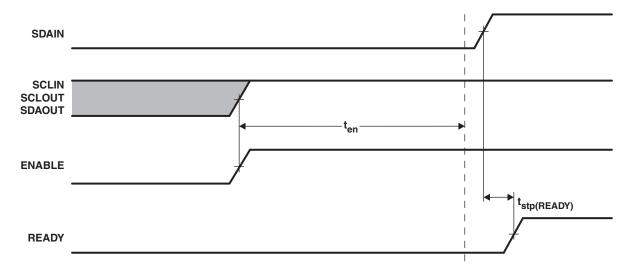
Figure 6.  $t_{stp(READY)}$  That Can Occur After  $t_{en}$
