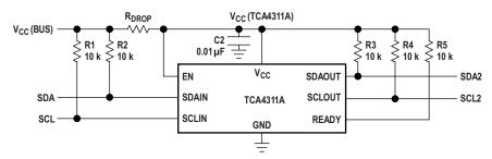
Figure 15. System With Disparate V<sub>CC</sub> Voltages Schematic
