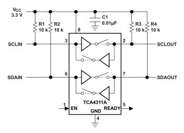
Figure 9. Application Schematic
