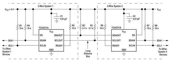
Figure 14. Repeater/Bus Extender Schematic
