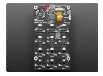
The red LED is located on the top edge of the back of the board, to the left of the USB connector.
