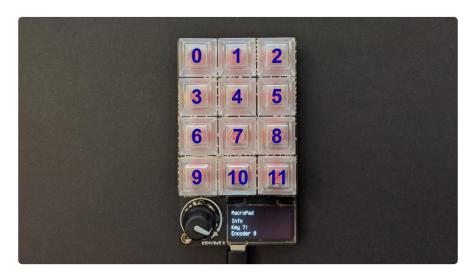
To rotate this example to 270 degrees, you would change the line of code from macropad = MacroPad(rotation=180) to the following:
