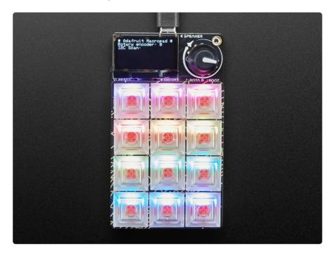
This space-ship is also fitted with a 128x64 monochome OLED for a crisp heads-up display that can be used in Arduino or CircuitPython to display keymaps, stats, computer performance, etc. There's also a rotary encoder with push-button soldered in. Twist and turn it or push to change volume or monitor brightness or scroll: whatever you like! A tiny speaker can give audio feedback or play fun bleepy tunes.
