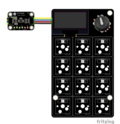
Simply connect the STEMMA QT cable from the STEMMA QT port on your board to the STEMMA QT port on the MCP9808.
