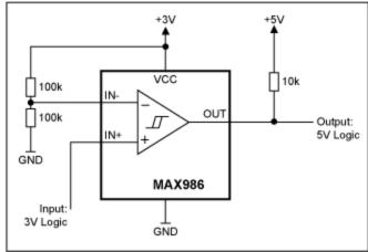
Figure 4. Level translation from 3V to 5V logic.
