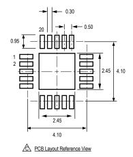
For Reference Only, not for tooling use (reference DWG-2864) Dimensions in millimeters Exact case and lead configuration at supplier discretion within limits shown
