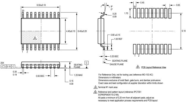
necessary to meet application process requirements and PCB layout tolerances; when mounting on a multilayer PCB, thermal vias at the exposed thermal pad land can improve thermal dissipation (reference EIA/JEDEC Standard JESD51-5)
