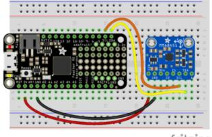
Board 3V to sensor VIN Board GND to sensor GND Board SCL to sensor SCL Board SDA to sensor SDA
