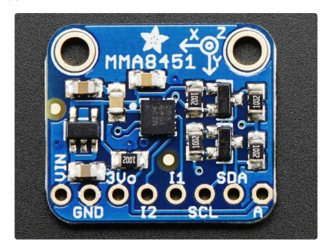
The little chip in the middle of the PCB is the actual MMA8451 sensor that does all the motion sensing. We add all the extra components you need to get started, and 'break out' all the other pins you may want to connect to onto the PCB. For more details you can check out the schematics in the Downloads page.
